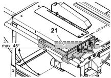
For use as mitre fence the short fence extrusion (21) must be installed. The mitre fence is mounted on a guide bar, fastened to the left-hand side of the saw table.
